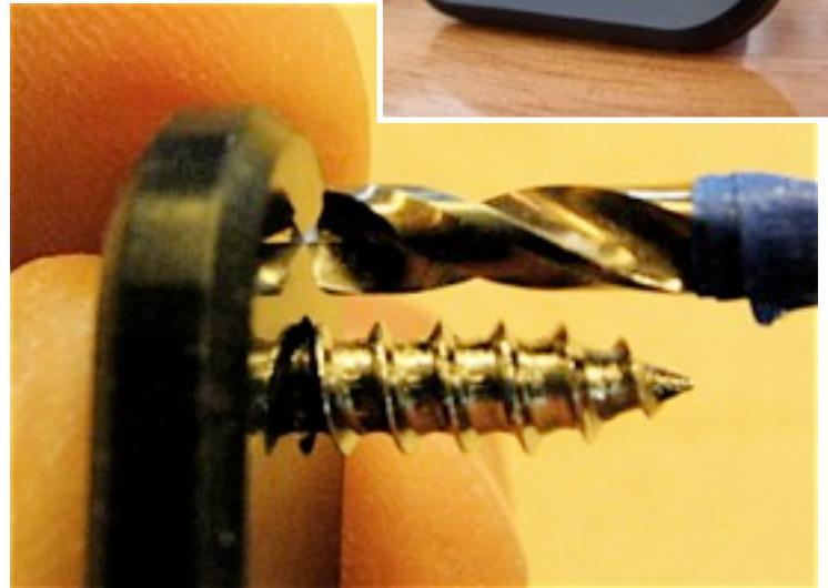
Drill the holes for the screws as square as possible to the surface and use a countersink to lightly bevel the edges of the holes.
