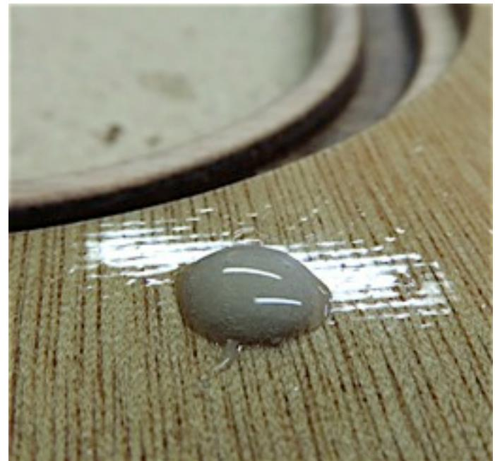
When cured, warm up the mounds of epoxy and slice them off flat with a sharp, wide chisel held flat. Push sideways on the chisel with your thumb to slice off the bumps (a bit at a time) and then lightly block sand to finish.
