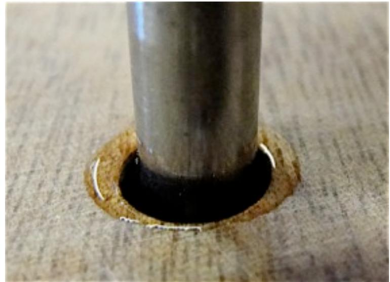
Add a small amount (the mix must pour) of 404 high-density fibers to epoxy to pour into the holes. Pinch the edge of the cup to make a spout. Leave a small mound of epoxy over each hole.
