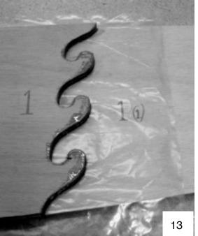
The next step is important to insure that the port and starboard panels are the same profile shape after gluing the puzzle joints:
