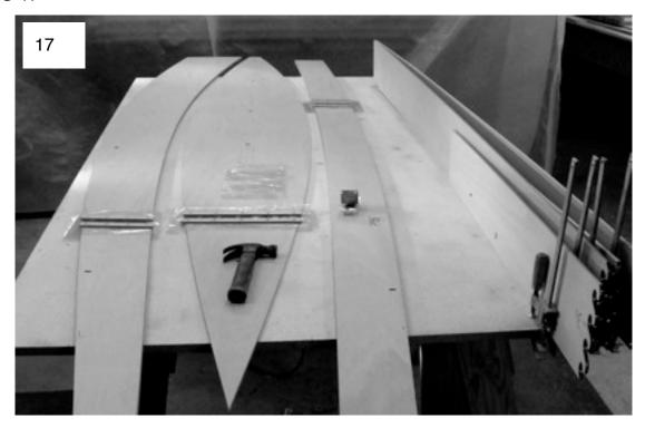
**Panels 3** will have to be placed elsewhere after applying epoxy to the joints so that the clamps can be removed from the bench to allow room for the panels on the bench.
