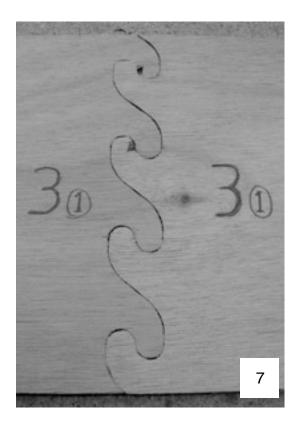
Proceed with marking and removing all the hull panels and stack them in the order that they will be glued (# 1 panels are glued first).
