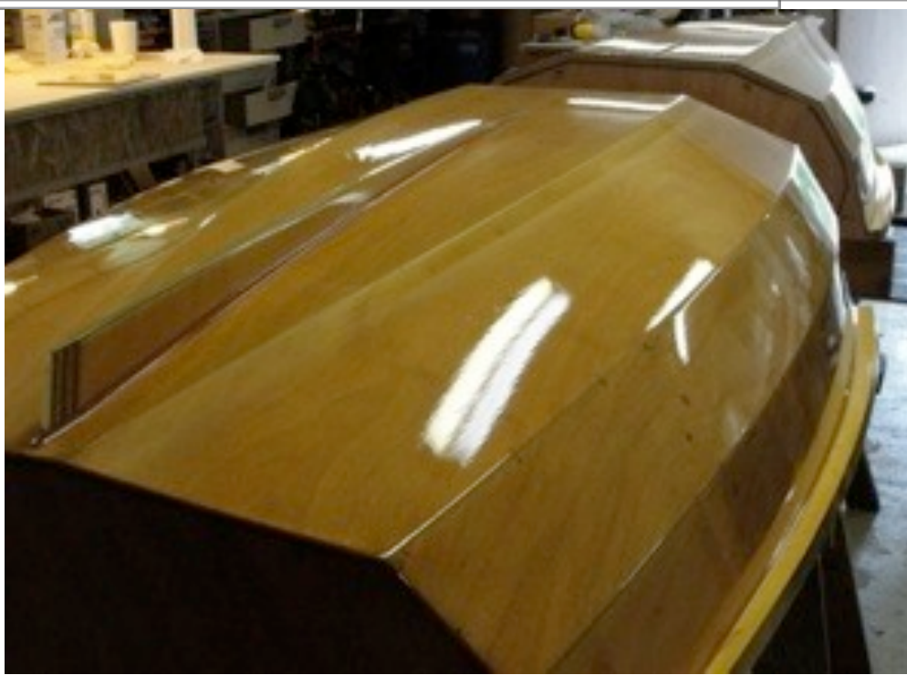
The hull halves fiberglassed and gloss coated.
