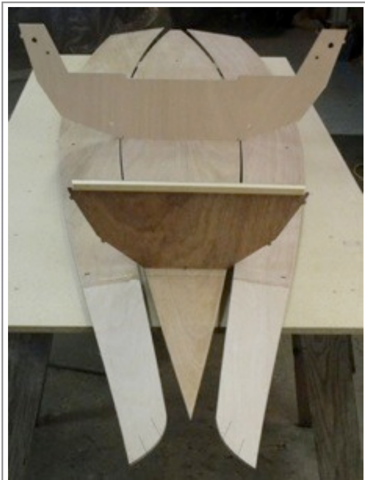
Assembling the hull by stitching the panels and bulkheads.
