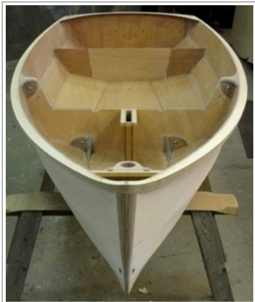
Main bulkheads, gussets, trunk, and mast partners installed.
