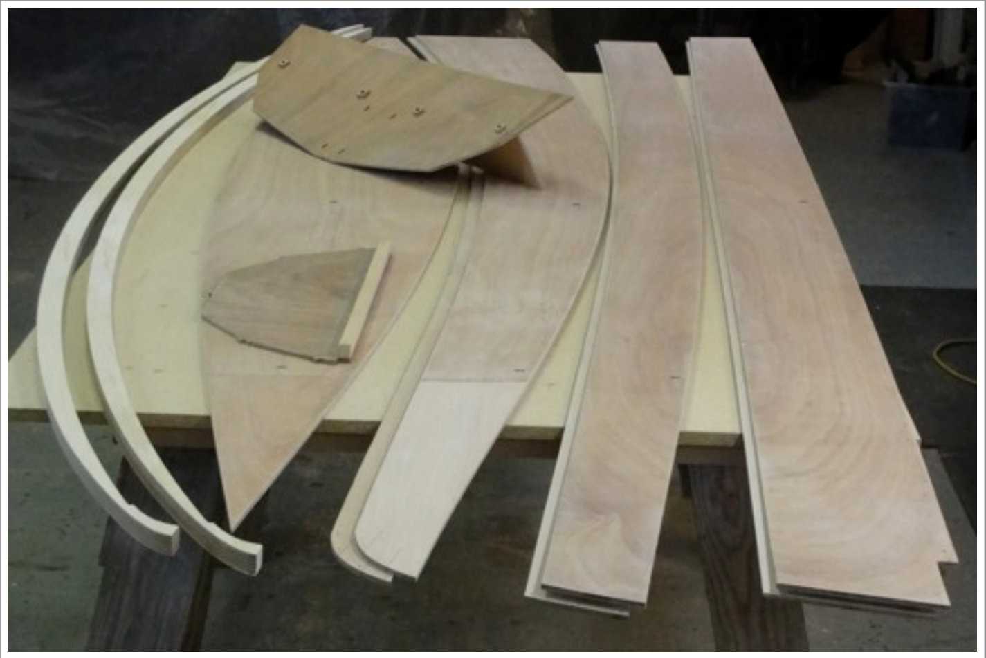
These panels have been assembled and pre-glassed as well as sanded in preparation for the next stage.
