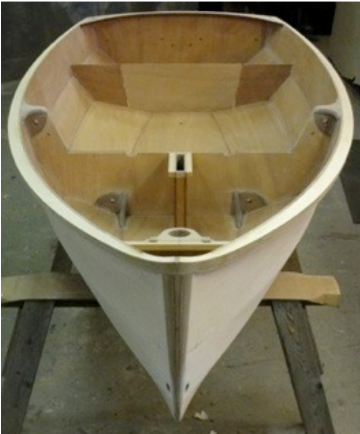
Main bulkheads, gussets, trunk, and mast partners installed.
