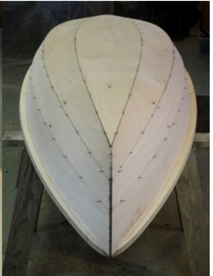
hull joints syringed with epoxy
