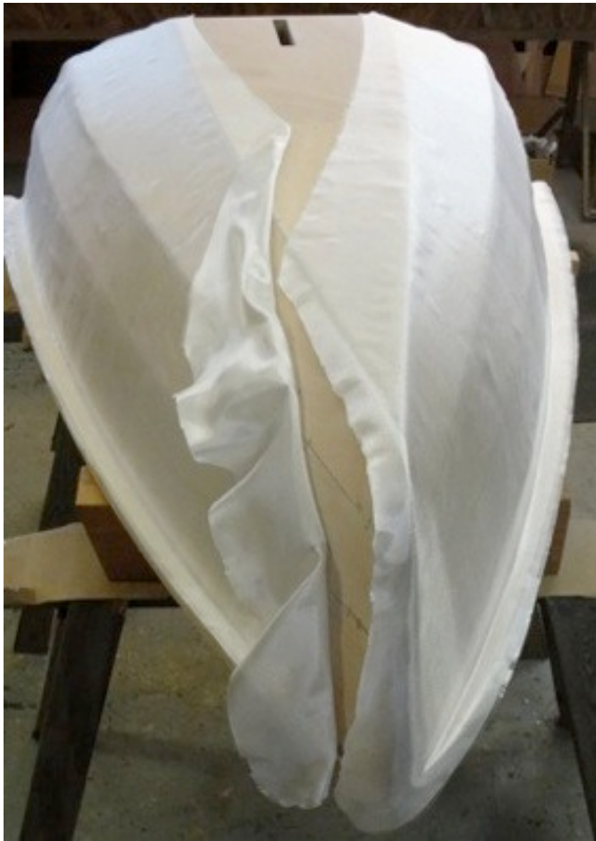
Fiberglassing the hull.
