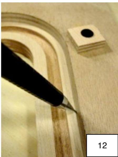
Turn the seat top over and mark around the coaming. Identify the orientation of the coaming, A-A, B-B, etc. PHOTO 13
