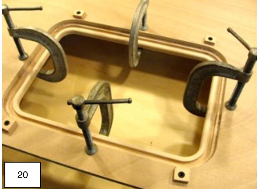
**The squeezed-out glue needs to be cleaned out completely or the lid will not fit.**
