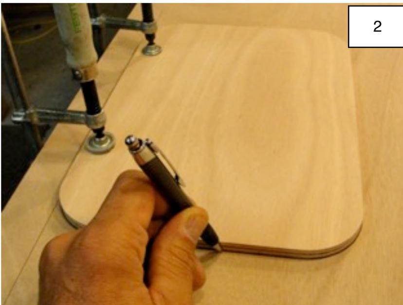
**Clamp the hatch lid to the seat top with one edge flush with the scribed pencil line** (fore & aft positioning is optional, just not too close to bulkheads). Trace around the hatch lid carefully with a ball point pen. Go around a couple of times for a clean, bold line. PHOTO 2
