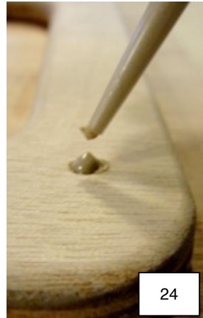
To make solid epoxy “plugs” for the turn dog fasteners, use the four screw holes (small hatch) to center larger holes. Use a **3/8”** (or so) drill bit marked with tape to drill holes to a depth of **3/4”**. PHOTO 25
