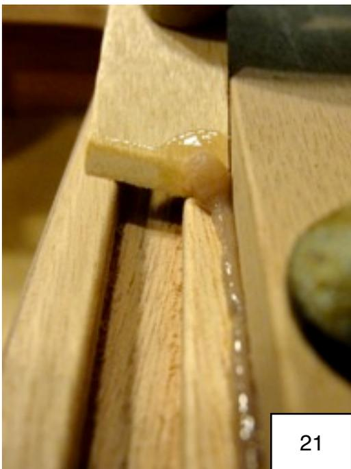
Push small bits of rag or paper towel on the end of a sharp stick to clean-up the last of the glue. PHOTO 22
