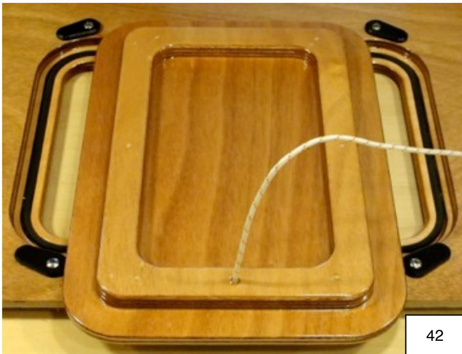
The lanyard can be attached to a hole drilled into the lid stiffener the same way. PHOTO 42
