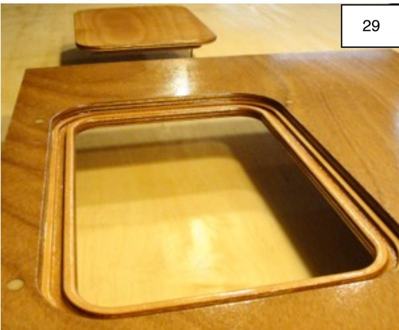
When applying the first coat of epoxy, start by applying a **very liberal coat to the gasket notch and cutout edge** with a brush. *Liberal* to insure that all that end grain plywood gets thoroughly coated. Next, **repeatedly dry the brush** on a clean rag and run around the notch and edge to **pick up all the extra epoxy**. PHOTO 30
