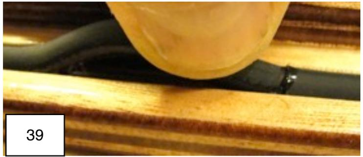
**The lanyard and and hatch pull loop** are made from the kevlar cord included with your hatch kit. The hatch pull loop should be centered at one end of the hatch and installed by drilling two **3/16"** holes an inch apart and **1 1/4"** from the edge of the hatch lid. Drill these holes **1/2"** deep and lightly bevel the edges of the holes with a countersink. PHOTO 40
