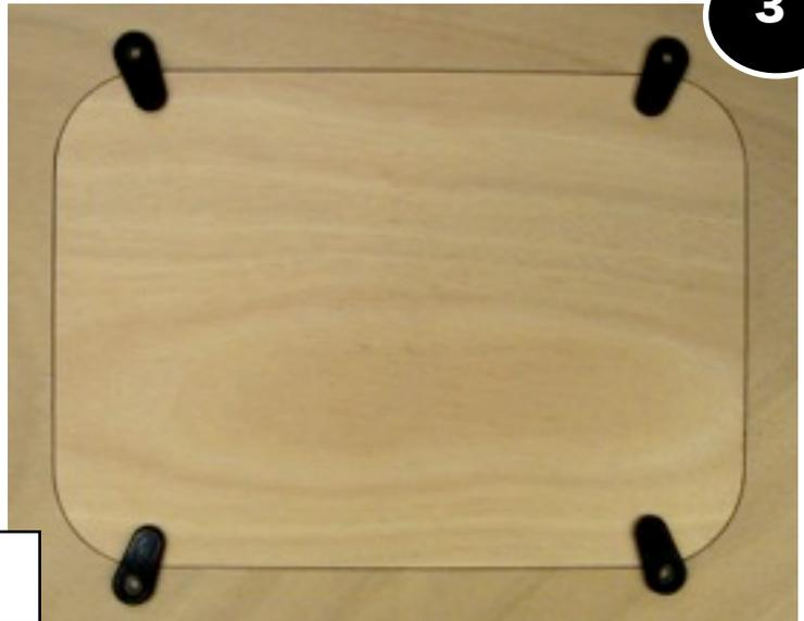
Use a straightedge to make pencil lines flush with the fore & aft (narrow) ends of the cutout. Mark lines parallel to, but 1 1/2" in from the first lines. PHOTO 7
