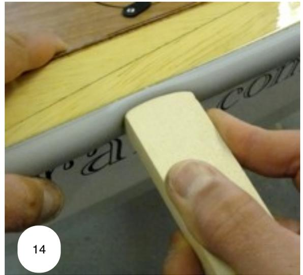
Once all the bumper sections have been installed and pressed down firmly, pull the tape and **use a firm eraser to remove any adhesive** that's not between the two parts. **This is much harder the following day.**
