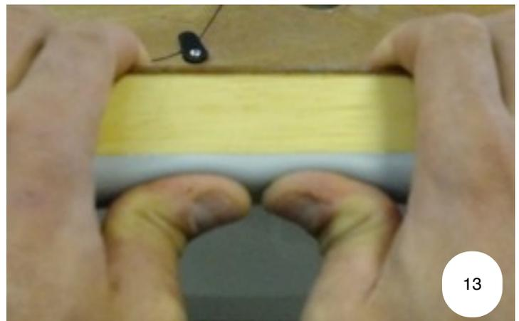
**Adhesion will be greatly increased by forcing the two glued surfaces together firmly** as soon as possible. One method is to round the end of a piece of wood and use it to firmly push the upper and lower edges of the bumper to the gunwale. PHOTO 14
