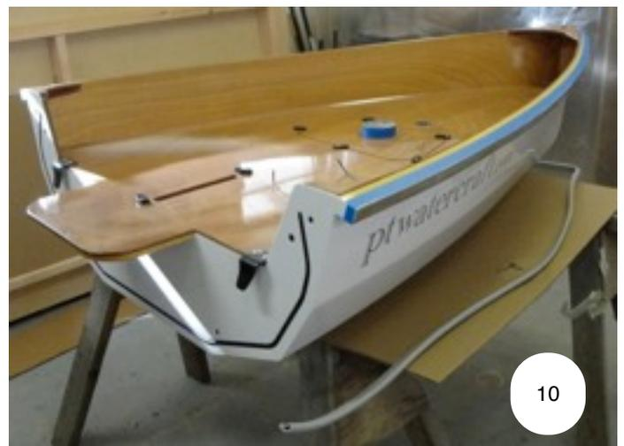
Hold a length of bumper out with one hand while using the fingers of your other hand (feeling above and below) to center the bumper one short section at a time.
