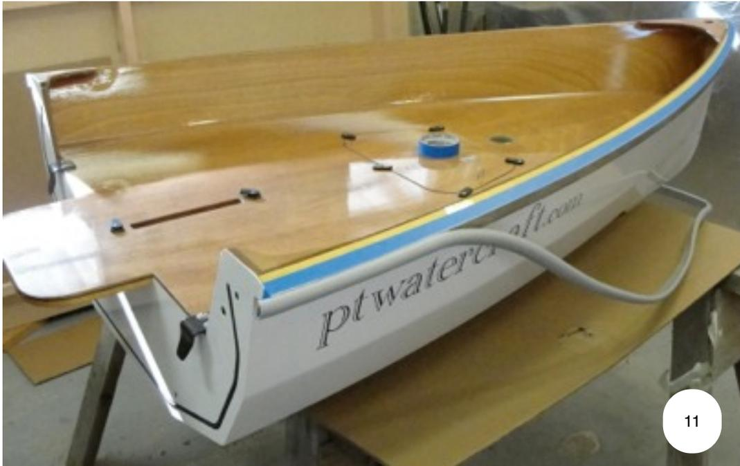
The flat side of the bumper should be about the same width as the gunwale, so using your fingers as a guide to get the bumper centered on the gunwale works well.
