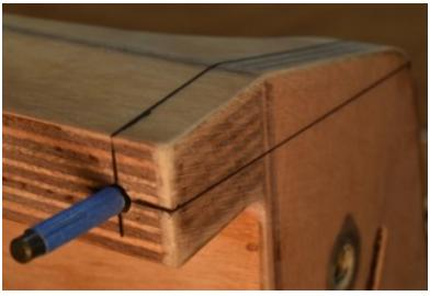
Use the pencil marks to align the drill when using the countersink. The recess should be deep enough for the head of the screw to be just below flush with
