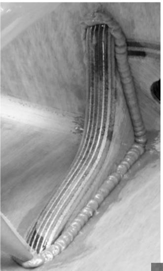
Start in the inside corner. When approaching the tip, lay the stick back at an angle to make the fillet bigger at the tips. Stop at roughly the middle of the tip and clean the stick.
