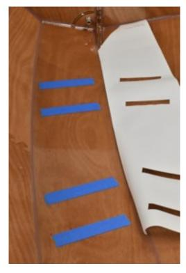
Hold each foot brace down firmly, centered inside the template cut-outs and mark around the foot brace with a sharp pencil (photo on left). Number as shown. Cut to the line with a sharp X-Acto® knife, light pressure, and a steady hand. Keeping knuckles or a finger
