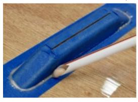
Clean-up is best done with a plastic straw with the tip snipped off at 45 degrees.
