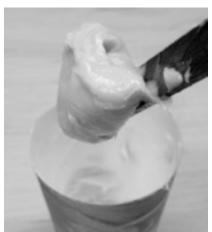
Apply more thickened epoxy than seems necessary to the lower gussets.
