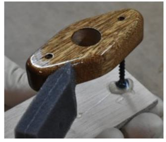
A small section of roller and a palette are by far the best way to coat the parts. The roller can apply an even film quickly. The tipping is done with a small 1" wide foam brush. Too much epoxy on these parts will cause drips (see next page).
