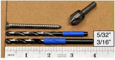
Mark a 3/16" drill bit to almost 1 3/4" as shown. This drill size will allow the screw to pass through the gunwale without threading.
