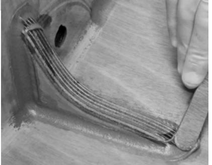
Clean up around the gussets is a challenge and must be done carefully, but it's much easier to do with the chisel stick than with sandpaper.
