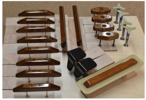
Pre-sand all the wood parts with fine paper (180 grit,or so) to remove router marks, etc. before mounting to the plywood strips.
