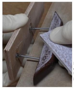
Apply epoxy evenly with the roller and gently tip with the foam brush, using very light pressure on the rounded edges.
