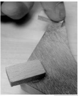
Cut and hot-glue on little plywood alignment blocks to the upper gussets. These 1/4" ply blocks should be about 1/2" x 1".
