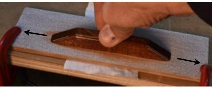
Sanding the flat faces of the braces is necessary. Because of the angle that the braces are placed on the curved hull panels it's a good idea to clamp the 1/4" thick sanding block over a strip or two of rag as shown to sand a reverse curve on the undersides of the braces. Use 80 or 100 grit and push firmly with short strokes (arrows).
