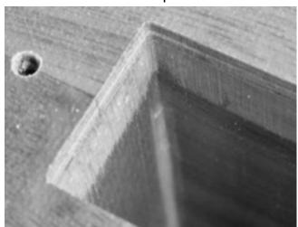
Apply a healthy saturation coat to the end grain of the plywood (hull bottom and foredeck) and then wipe up the excess with paper towel. This can be done with a gloved fingertip or a glue brush, but wipe up all the excess epoxy. Sealing the edge grain will prevent bubbles from forming under the strips. Let the epoxy cure and then give the edges a light sanding and 3-M scrubbie, or you can glue in the strips later the same day if the parts are pre-cut and fit and the temperature is cooling.
