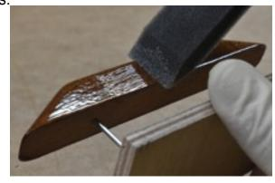
Note: there is some advantage to applying the final coat to the foot braces after installation. It's easier to tape the hull around the foot braces (for coating) than it is to tape the foot braces for gluing. See page ???
