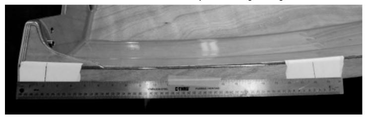
Set the combination square at to 13/16" (3/4" plus 1/16") and make marks parallel the the outer edge.
