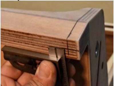
While the holes and screws don't need to be perfectly aligned, lines should be drawn in pencil to provide a guide for drilling.
