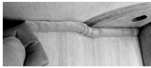
The gap at the beginning of the fillet is fine, it gets filled when filleting the gussets.
