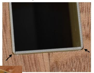
Lightly round the lower (inside) edges of the strips with a sanding block.
