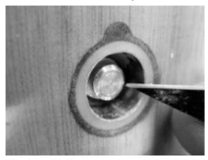
Bevel the edges of the holes with a **countersink** until you see metal all the way around.
