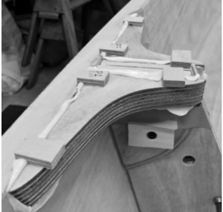
To avoid breaking off the alignment blocks when gluing the upper gussets, press down on the tips of the blocks (not the gusset) with your fingers when pushing the gussets into the corner as shown.
