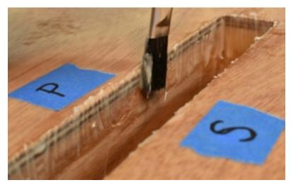
Because the strips are transparent, you will be able to see the glue squeezing out when the strips are pressed in place. **The goal is to avoid much squeeze-out at the bottom** (inside) edges, so start by pressing near the bottom edges to force the glue upward.
