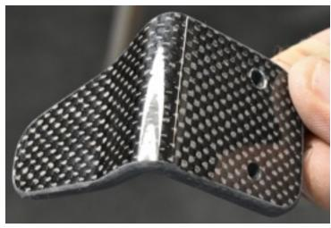
Apply the coating on the clips thin (even if it takes two coats) to avoid drips and maintain the angles on the outboard edges (where the clips touch the bulkhead edges).
