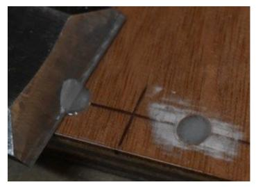
Mark a 1/8" drill bit at 3/8' as shown and drill all holes to that depth square to the surface. Using a fresh driver bit (or screwdriver) will insure that the screws are started square to the surface. Trial fit all screws and eye straps.
