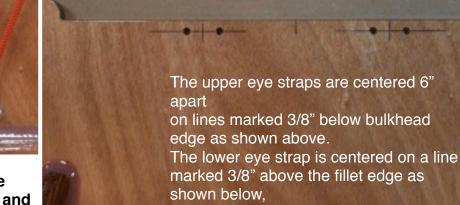
The eye straps can be centered on the lines and holes marked with an awl as shown below.
