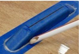
Clean-up is best done with a plastic straw with the tip snipped off at 45 degrees. Clean up enough to see that the cleat is centered inside the tape, press down more firmly and clean again. Pull the straw through a folded rag to remove goo.
