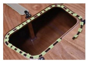
The trunk cap gasket is much easier. Tape the gasket in place with the white dots facing down. Carefully cut the butt joint about 1/16" over length and compress into place.
