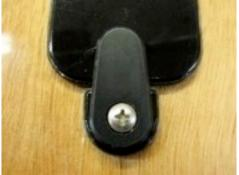
Back the screws out and apply a tiny amount of epoxy to the inside of the holes with the tip of a nail or drill bit. Install and tighten the screws. Back off on the screws until the dogs turn with a small amount of friction and allow the epoxy to cure.
