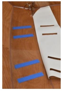
Hold each foot brace down firmly, centered inside the template cut-outs and mark around the foot brace with a sharp pencil (photo on left). Number as shown. Cut to the line with a sharp X-Acto® knife, light pressure, and a steady hand. Keeping knuckles or a finger pressed to the hull can help in following the line.
