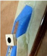
Squirt thickened epoxy all the way through the screw holes with a syringe. Use a bit of 407 filler to color match and leave a small mound of epoxy over the holes.
