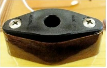
Turn the hull over and inject the holes around the sockets with a fresh batch of un-thickened epoxy in a syringe.
