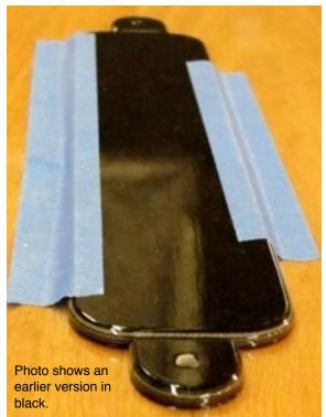
The two little riser pads can be glued on without sanding the foredeck. Acetone wipe the foredeck and sand the undersides of the pads. **Apply a thin film of un-thickened epoxy** to the undersides of the pads and push into place with a small gap between the cap and pad. Center the pads using the joint in the foredeck panels as a centerline. Note: insert the butt end of a 3/16" drill bit into these tiny parts for applying the film of glue and twist the bit out while holding them in place.
