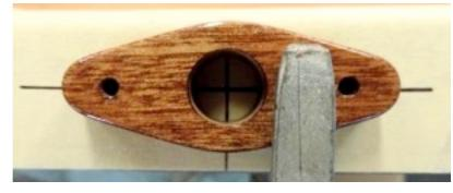
While the block is clamped, **pencil mark around the block** and **identify as shown** on right and next page. Carefully cut to pencil marks and remove tape.
