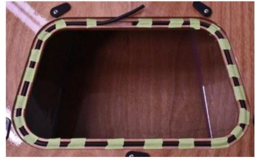
Rub the tape down firmly to the gasket as it will stay attached and help keep the upper face facing up when gluing.
