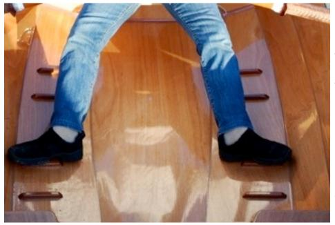
Our personal boats have been set up for a 6' rower and a 5' 2" rower. The template that we provide for placing foot braces is based on these heights. The 5'2" rower is using the aft oarlock sockets in the photo below.
