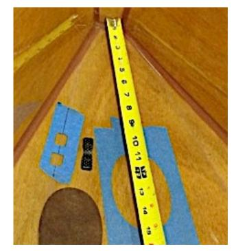
Scrub bond area thoroughly with 3-M scrubbie. Sand the bottom face of eye strap on a sanding block. Wipe clean. Glue with gluing fillers after a thin finger-tip prime (or use G-flex epoxy). Press the eye strap in place and clean epoxy from eye strap (onto tape) with a chisel stick.
