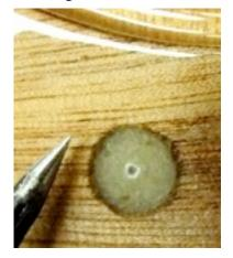
Drill the holes for the screws as square as possible to the surface of the foredeck and use a countersink to lightly bevel the edges of the holes.
