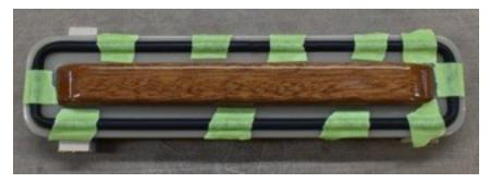
Carefully pull up the side of the gasket without the butt joint.
