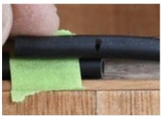
**Cut the end off square** using a thin scrap of wood to cut on and following inst. on previous page.
