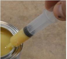
Stir the contact cement and suck up about half a syringe full with a new syringe.
