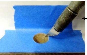
Tape over the bottom ends of the holes and knife out with an X-Acto® knife. Add tape to the hull for dripping epoxy.
