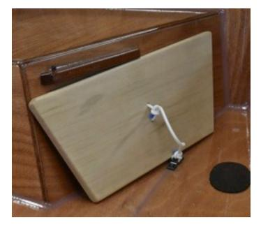
The back seat needs "stops" to keep it from sliding forward. We now make these from 1/4" black fiberglass rod. The stops are tiny, but the ends can be easily rounded by chucking one end up in a drill and sanding the ends while spinning.
