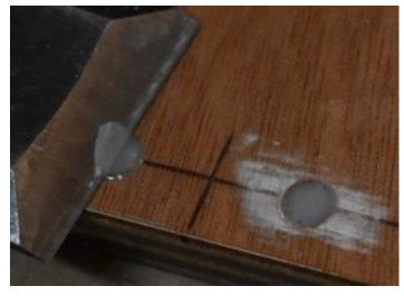
Mark a 1/8" drill bit at 3/8' as shown and drill all holes to that depth square to the surface.
