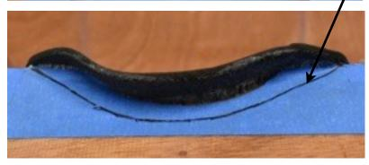
It may be necessary to tape the outboard corners down tightly until the contact cement cures.
