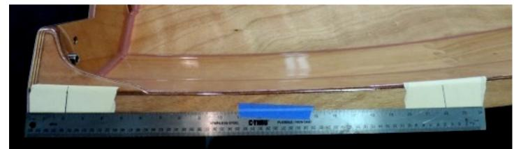
Set the combination square at to 13/16" (3/4" plus 1/16") and make marks parallel the the outer edge. **Note**: the tape doesn't wrap over the outboard edges.
