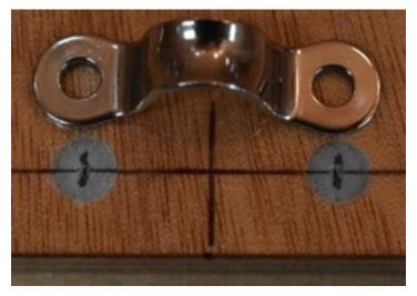
Fill the holes with un-thickened epoxy and install screws and eye straps. Drive screws slowly to allow epoxy to spiral up around the threads to avoid hydraulic pressure damage.
