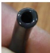
Apply cement to the remaining notch, tape down most of the gasket and then syringe just a bit of cement to the tip of one end as shown.
