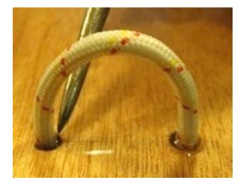
The lanyard can be attached to a hole drilled into the lid stiffener the same way. The lanyard should be about 2 1/2 feet long. One end can tie around the mast tube. The other can be glued into the lid stiffener on the under side of the hatch, on the forward edge, on centerline, in the same way we describe above.
