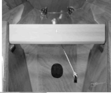
The back seat can slide between the eye strap and the seat cleat. It should wedge snug enough to stay out of your way when nesting. You may need to trim your seat very slightly narrower for this to work.
