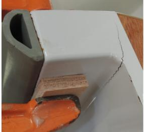
The trick for gluing the crack is to drill a hole at an angle that intersects the crack and have the hole and the tip of the syringe be the same size. Cut off the tip of the syringe until it just fits the outside edge of the hole that you drill.
