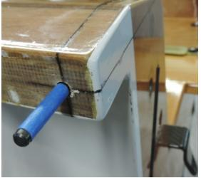
Countersink the hole deep enough that the head of the screw can be well below the surface. This will allow filling (with epoxy) over the head of the screw for a reliably watertight seal.
