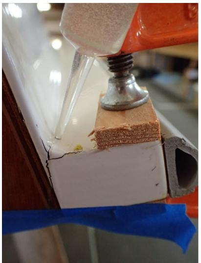
The screws pass through the gunwale without threading and then thread into the bulkhead and gusset. When tightened, the screws will pre-load the failure area and make another failure very unlikely.
