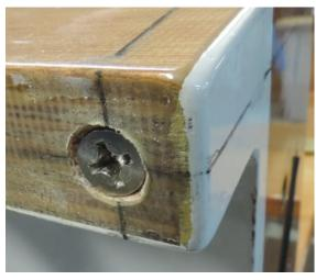
We stood the hull half on one edge and then the other for installing the screws.
