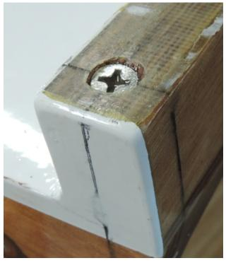
We used hypalon glue to re-attach the bumper ends after thoroughly sanding both surfaces and wiping with clean rags.
