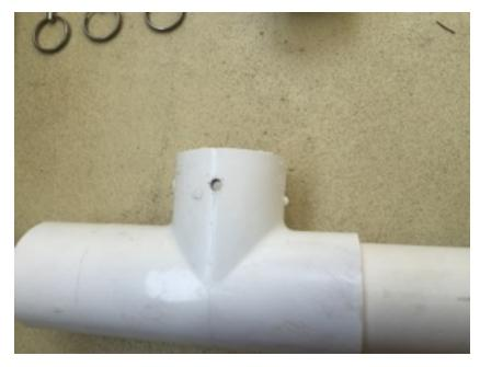
It is constructed with PVC glue, and the bottom axle part is epoxy/silicone caulk sealed on the inside to prevent it from filling with water when launching. There are 2 jam nuts on either end of the axle tightened against the PVC caps to hold the axle on center and prevent it from spinning in the PVC housing while tightening the wheels on with the wing nuts.
