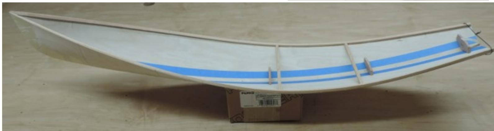
My first two attempts broke (very loudly) on the keel line using just a bead of epoxy. The latest model uses a 1/2" wide strip of 4 oz cloth with a bead of epoxy over it. This puts the glass in tension and the epoxy bead in compression. This seems reliable but a full cure is necessary before folding.
