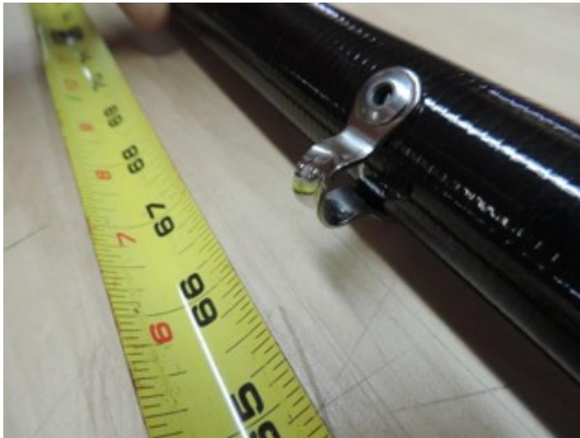
Mid way from the above block and the aft end of the boom, the main sheet runs through a fairlead made from a re-shaped eye strap. This is also on the lower side of the boom.
