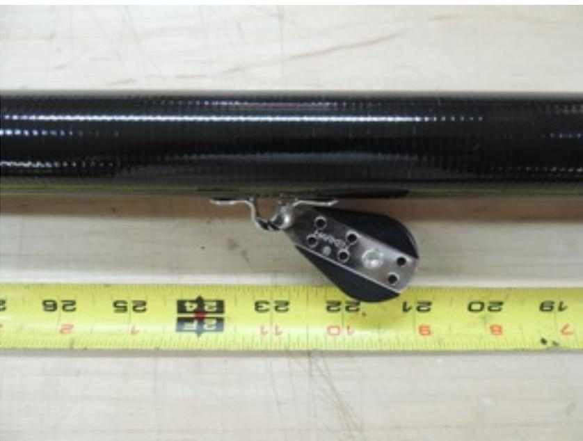
Eye strap with block attached to the **lower face of the boom 23"** aft of the forward end of boom.
