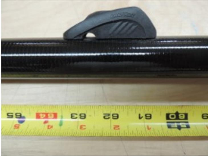
The sole becket block for the main sheet can be attached by lashing as shown.
