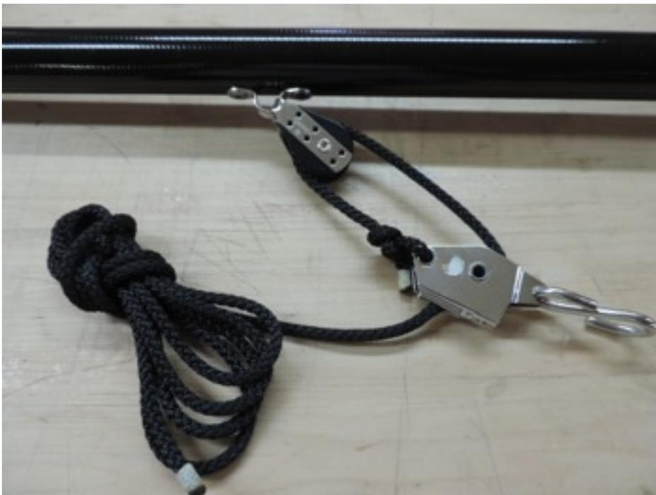
Vang set up as shown with vee jam cleat facing down.
