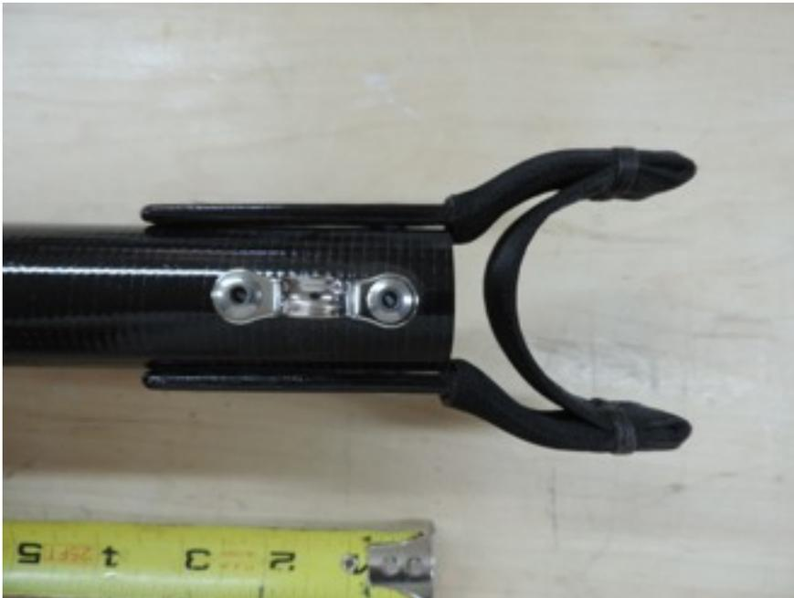
**The tack eye strap is attached to the upper face of the boom with the shorter rivets, forward hole 1/2" aft.**
