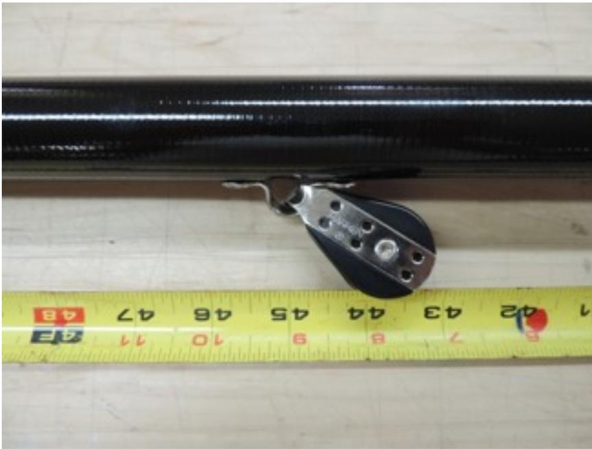
Eye strap with block attached to the **lower face of the boom** at 45" aft.
