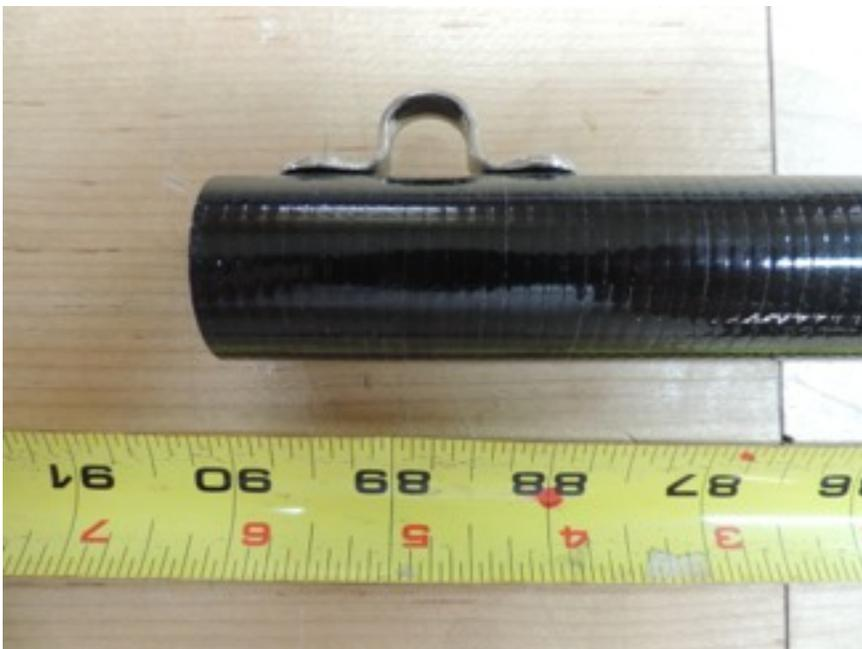
At the aft end of the boom **on the upper face**, an eye strap for the outhaul to run through. Aft hole no closer than 1/2" from end of boom.
